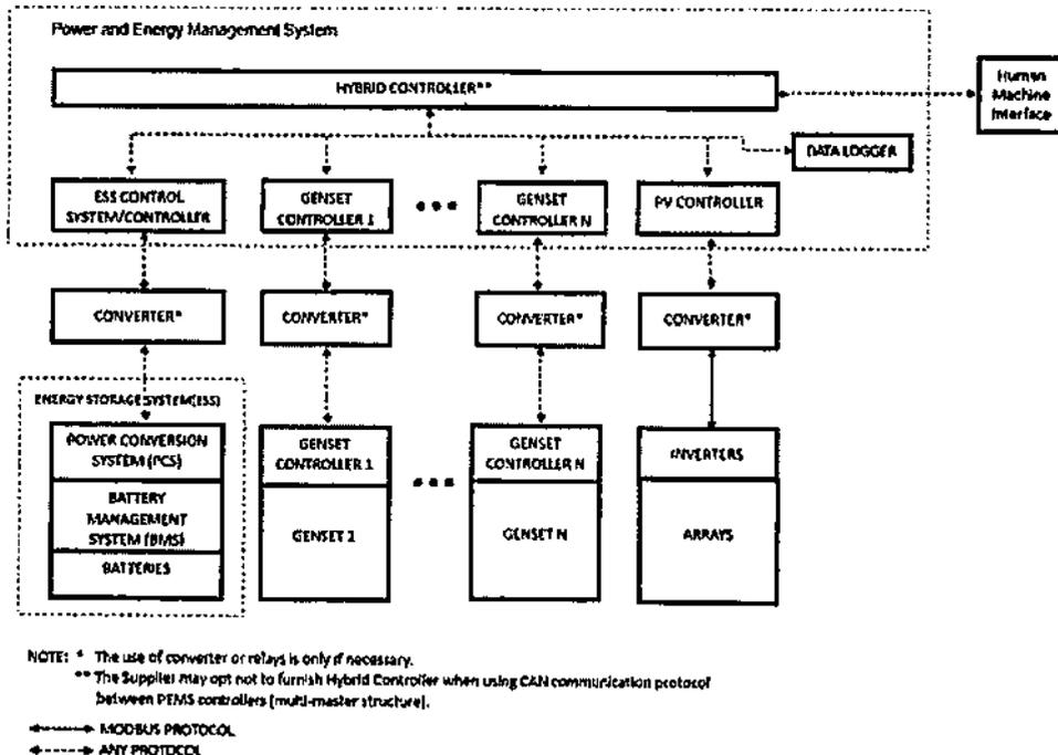
Figure 1: PEMS and Communication Diagram
